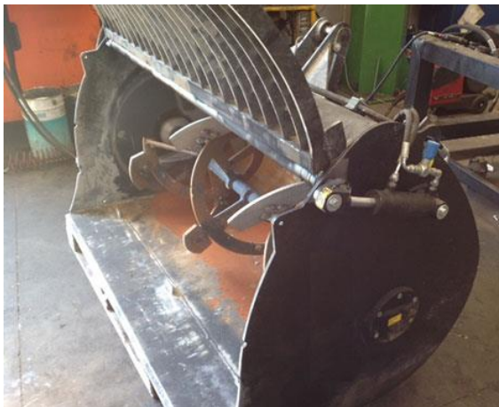
Left: Hungry Pig "Mix and Load" powered bobcat attachment designed to scoop bulk materials, then tip food waste bins directly into the mixing bucket and engage the mechanism to size reduce and mix material to form a suitable feedstock for composting. Image source
